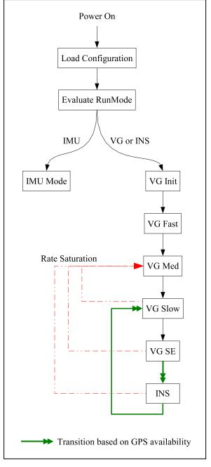
must be configured for INS operation (which is the default) and GPS must be available. The MIDG II will not transition into INS mode without GPS. The MIDG II will remain in INS mode until the accuracy of its estimates
